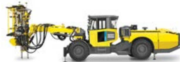
Underground production drill rig equipped with smart automation functions for higher equipment availability and enhanced overall productivity
