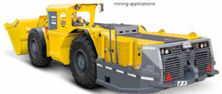
Battery-driven underground loader for mining applications
